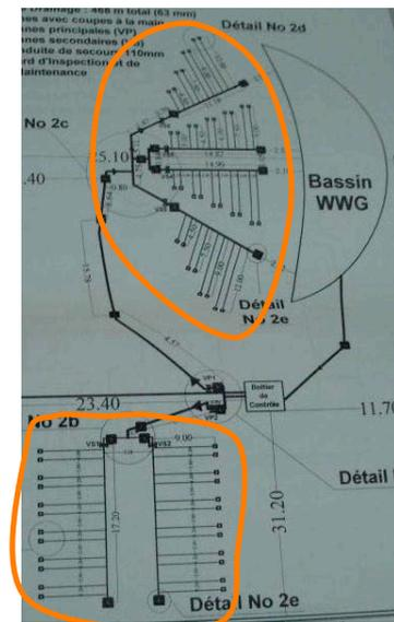
Figure 7d. Plan of the WWG unit's drainage system: 468 meters drainage in 2 major areas (orange lines) and 6 sub-sections, gravity flow.
