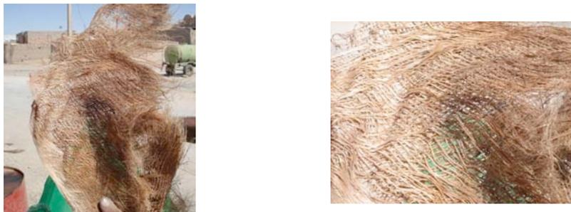
Figure 7b. Close-up of the local material used for the filter at the exit of the sewage water of the primary treatment.
